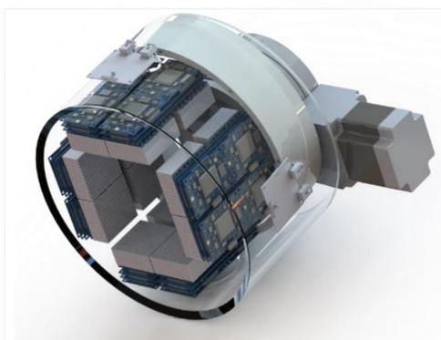
Fig.1. CAD design of the Proposed high-resolution PET scanner.
