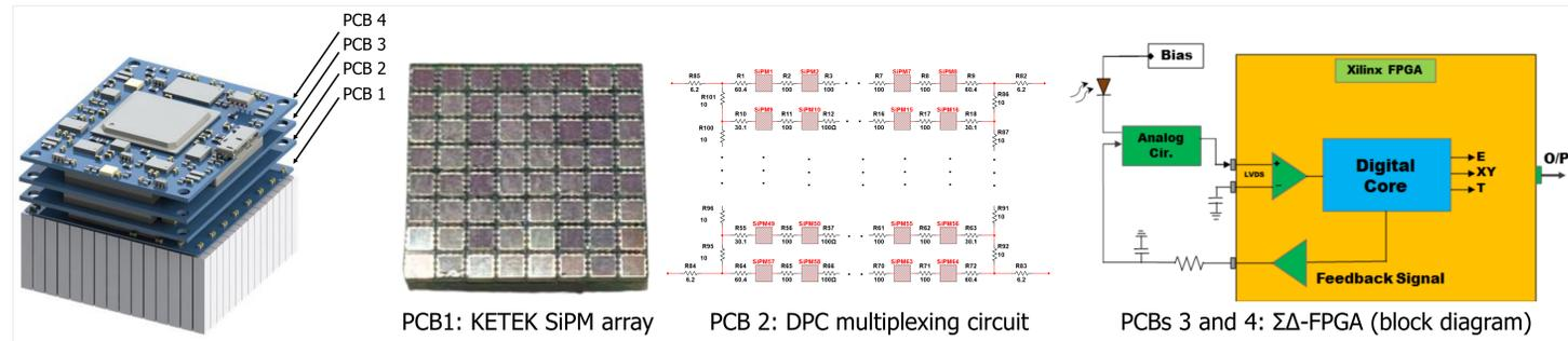
Fig.2. Left: Modular PET detector, PCB1: KETEK SiPMs array, PCB2: DPC multiplexing circuit, PCB 3&4: ΣΔ-FPGA block diagram.
