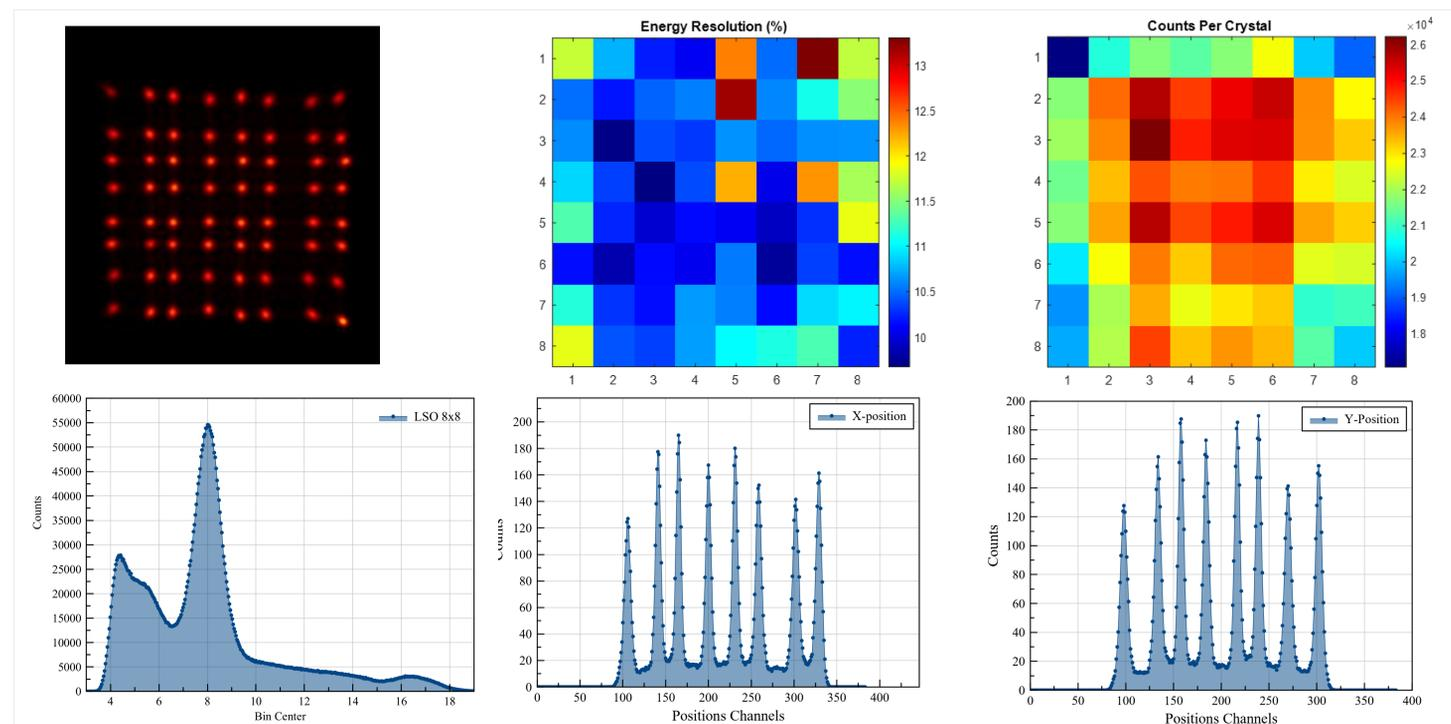
Fig.3. Top: Flood histogram map of PET detector (Left), color-coded map for energy resolution (Middle) and counts (Right) per crystal. Bottom: Energy resolution histogram for the array (Left), X-position profile (Middle), and Y-position profile (Right).
