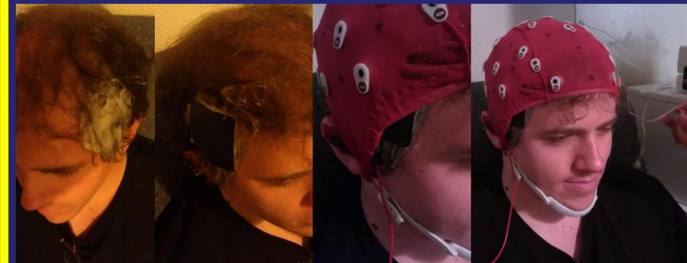
35 cm<sup>2</sup> electrodes, alcohol, conductive paste + gel, 64 ch EEG cap
